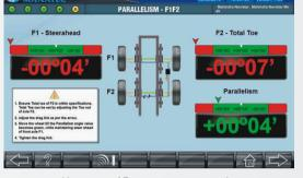
Alignment of Front twin steering axles
