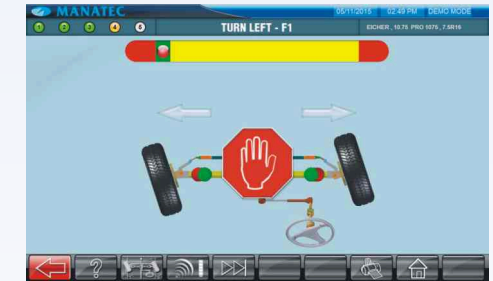
Screen guidance for Turn Left & Right to measure Caster & Kingpin inclination
