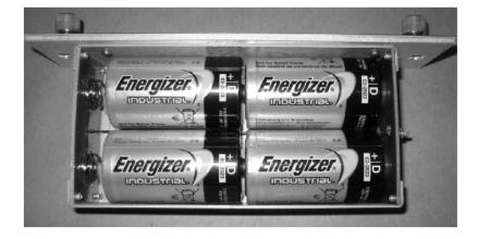
Replace the battery box and tighten thumbscrews.
