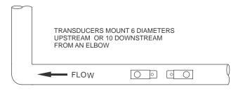
TURBULENCE INCREASING DEVICES: Elbows, flanged connections and tees tend to introduce desirable conditions of an evenly distributed flow profile. Transducer mounting 6 pipe diameters upstream and 10 diameters downstream from these disturbances is generally optimum.
