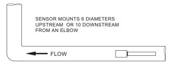
Turbulence Increasing Devices: Elbows, flanged connections and tees tend to introduce desirable conditions of an evenly distributed flow profile with some air or gases entrained in the flow. Sensor mounting 6 diameters upstream and 10 diameters downstream from these disturbances is generally optimum.
