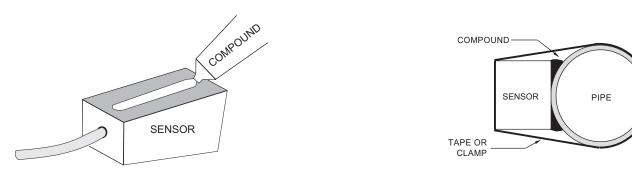
For proper operation the transducer must be fixed securely to the pipe with coupling material between the transducer face and the pipe. Sensor installation with excessive coupling compound or use of epoxy can result in gaps or voids in the coupling and cause errors or loss of signal. Insufficient coupling compound will create similar conditions.
