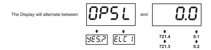
The Output Simulation function controls the digital display 4-20mA output and control relay. Use it to simplify calibration of remote 4-20mA devices such as chart recorders or remote displays, and to test relay set-points.
