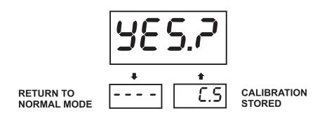
Press ★ to Store calibration (LIT will display -**C.S**-). Calibration is stored in non-volatile memory (even through power interruptions).
