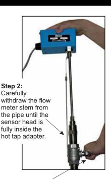
Step 3: After the meter is completely withdrawn, slowly close the valve to isolate flow.
