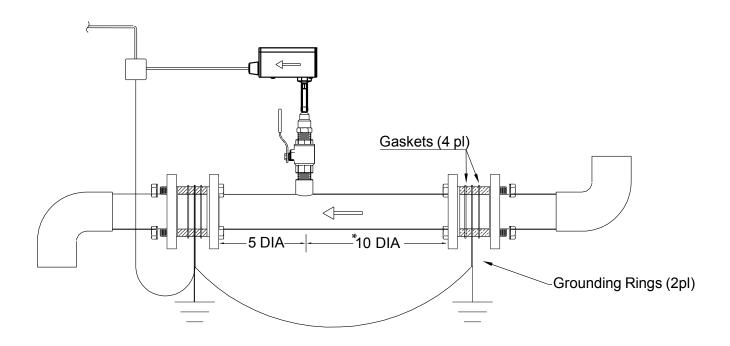
\* Additional straight run may be required upstream of the upstream grounding ring based on the nature of the upstream obstruction. Refer to the chart in Section 3.1 on page 11 of this manual to determine how much straight run is required.
